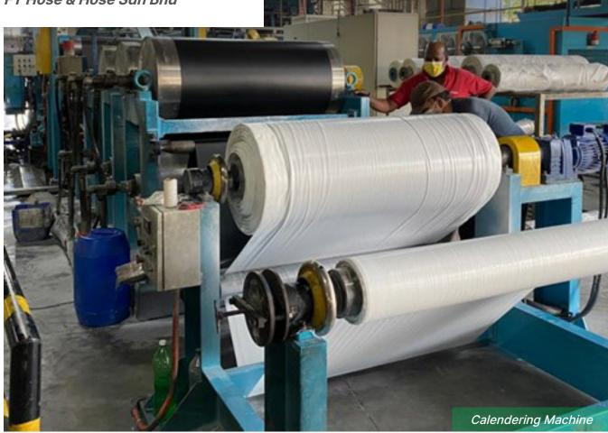
FT Hose & Hose Sdn Bhd enhanced its production processes by implementing advanced calendering and lathe technology to enhance efficiency and improve product quality. With the assistance of the FAGT, the company invested in an automated calendering machine, enabling in-house production of rubber fabric compound sheets. This strategic move has resulted in a remarkable 20% improvement in product delivery compared to purchasing fabric from local suppliers.
